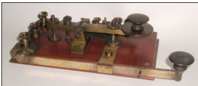
A morse code key identical to that used on the Titanic. Keying the “spark gap” transmitter could fuse the contacts together. The long brass lever was an emergency disconnect should this occur.
