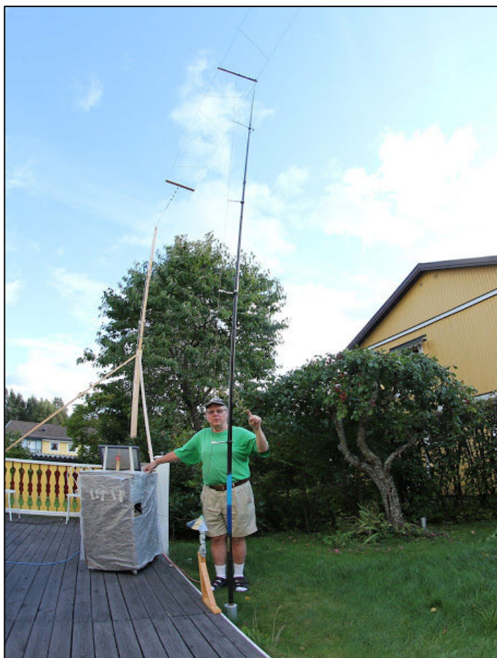
Figure 1 - Sven, SM5LE with receiving equipment. In front of Sven is his vertical antenna for receiving the Schumann resonances' electric field part. The big box contains an amplifier, built with a single transistor. The amplifier feeds his indoor PC sound card. The amplifier is battery operated and the battery is charged by solar power.
