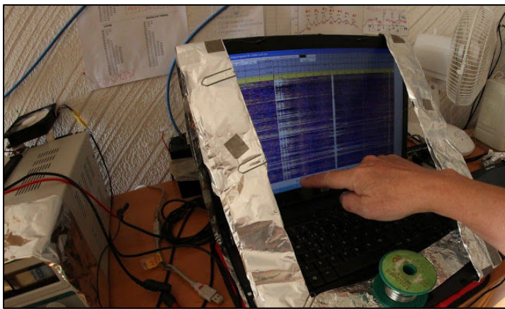
Figure 2 - Sven points the trace of a Schumann resonance at 7.83 Hz. His attic is almost occupied by a loop antenna, which is near completion for receiving the magnetic field part of Schumann resonances.
