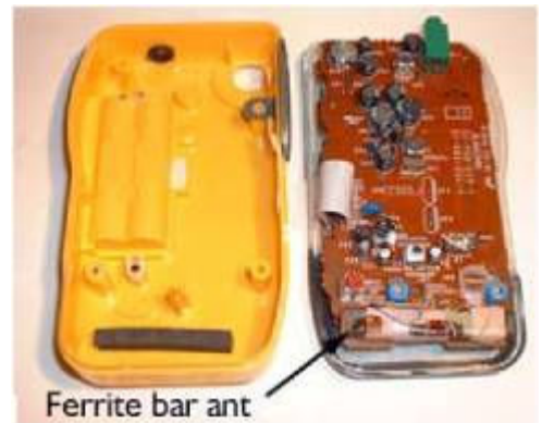
The ferrite bar antenna in a portable AM radio can be helpful in locating sources of interference.
