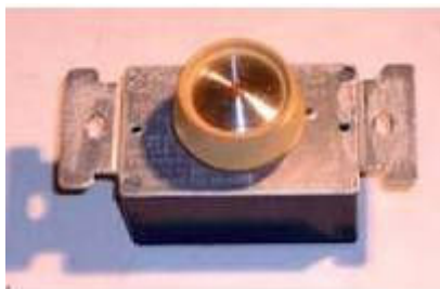
Thruster-based light dimmers can generate lots of noise at MF and HF. They are best avoided.
