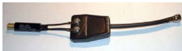
Two TV antenna matching transformers connected back-to-back can make a ground loop isolator.
