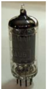
7-pin all-glass vacuum tube (6AU6)
